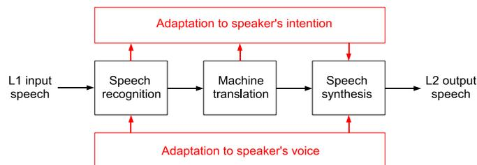
Figure 1: The black parts are a traditional S2ST system. EMIME added the lower path in grey; SIWIS will focus on the upper path
